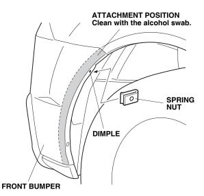
3. Locate the dimple in the front bumper. Slide a spring nut over the dimple.
