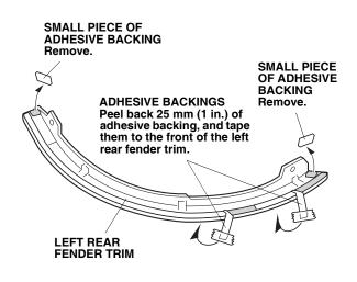
34. Position the left rear fender trim on the left rear fender as shown.
