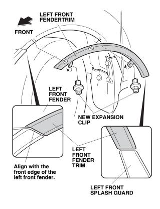
16. Slowly and carefully peel the adhesive backings from the left front fender trim. After removing all of the adhesive backings, press the left front fender trim firmly against the left front fender with the palms of your hands, particularly at the ends, for 30 seconds.
