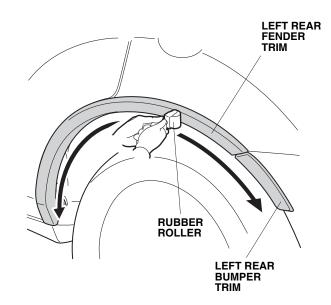
Repeat steps 1 through 39 to install the fender trim 40. on the right side of the vehicle (Turn the steering wheel all the way clockwise in step 8).
