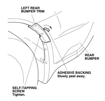
28. Tighten the self-tapping screw installed in step 26.
