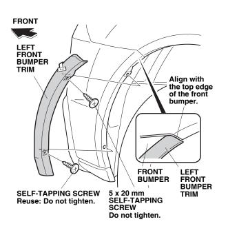
6. Slowly and carefully peel the adhesive backing from the left front bumper trim. After removing the adhesive backing, press the left front bumper trim firmly against the front bumper with the palms of your hands, particularly at the ends, for 30 seconds.
