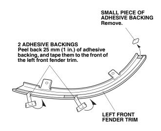
15. Position the left front fender trim on the left front fender, and align it with the front edge of the left front fender. Install two new expansion clips through the left front fender trim.
