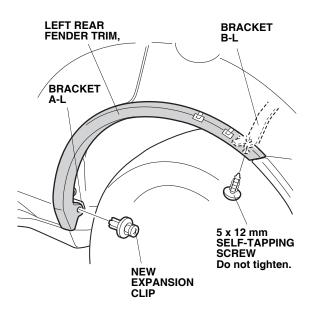
While pushing up on the left rear fender trim, 37. slowly and carefully peel the adhesive backings from the left rear fender trim. After removing all of the adhesive backings, press the left rear fender trim firmly against the left rear fender with the palms of your hands for, particularly at the ends, for 30 seconds.
