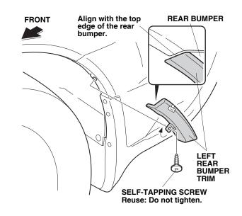
27. Slowly and carefully peel the adhesive backing from the left rear bumper trim. After removing the adhesive backing, press the left rear bumper trim firmly against the rear bumper with the palms of your hands, particularly at the ends, for 30 seconds.
