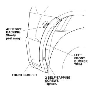
7. Tighten the two self-tapping screws installed in step 5.
