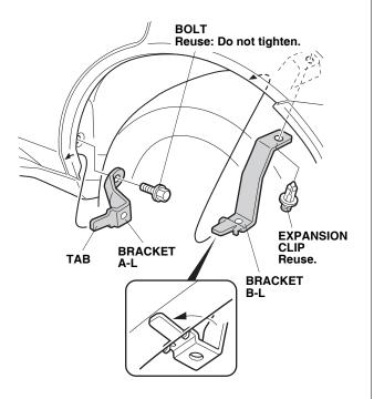
32. Install bracket B-L using the expansion clip.
