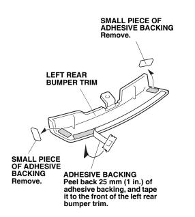
26. Position the left rear bumper trim on the rear bumper, and align it with the top edge of the rear bumper. Install the self-tapping screw through the left rear bumper trim, but do not tighten it yet.
